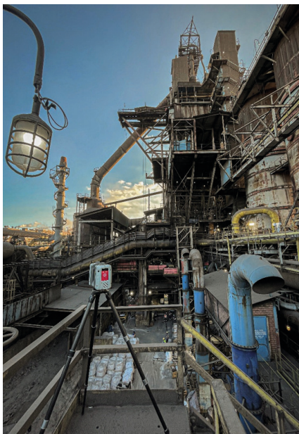
Fig.6. Scanning survey of a steel mill.
