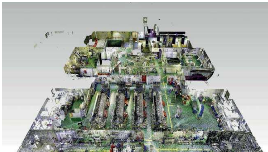
Figure 3: Scanned engine and pump room
